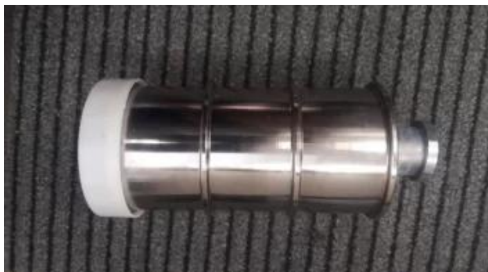
AAA20780A1 Shave L-255mm 3 grooves Pitch=65mm for OTIS GEN2
