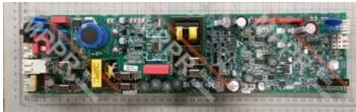
GCA26800PM10 LVPB 230 V AC power supply PCB
