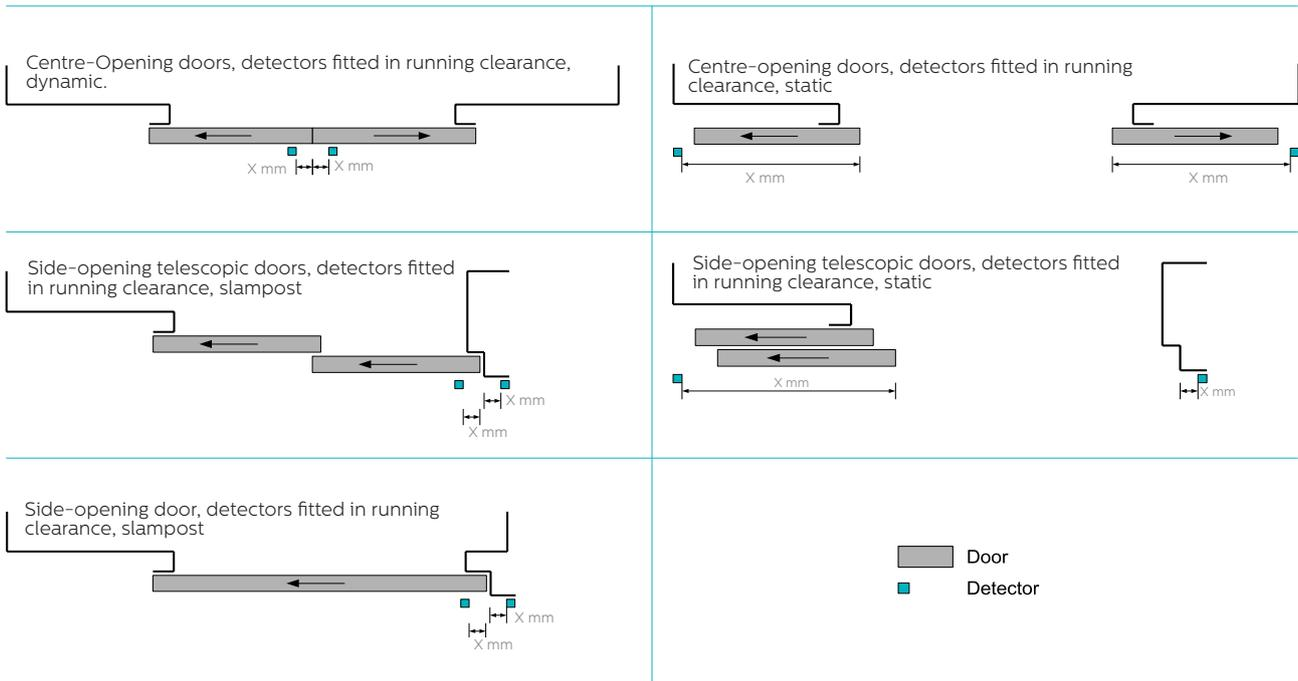
Light curtains with diode spacing greater than 50mm can still comply with EN81-20 when installed at some set back distance from the edge of the elevator door. This guide shows how E10 20 can comply with EN81-20 in specific installations.
