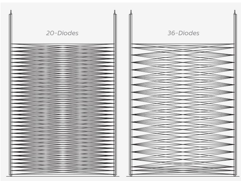
Fig 5: Diode beam pattern for 20 and 36-diode detectors
