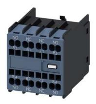
auxiliary switch, on the front, 2 NO + 2 NC, 53/54, 61/62, 71/72, 83/84, current path: 1 NO, 1 NC, 1 NO, spring-loaded terminal, physically coded, only with contactor relays 3RH2140 and 3RH2440 combinable (according to EN 50011)
