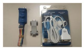
Connection cables set for MP test tool
