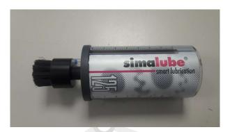
Oil lubricant with brush SIMALUBE SL14 125mm
